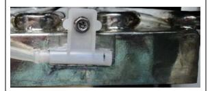
As soon as the pan starts to open the defrost backup timer starts, if the thermistor mounted on the evaporator does not reach the defrost completion temperature before the timer times out at 30 min. the display will show "E2" and the unit stops. (if the HGV does not open this could also give you an "E2" error)
